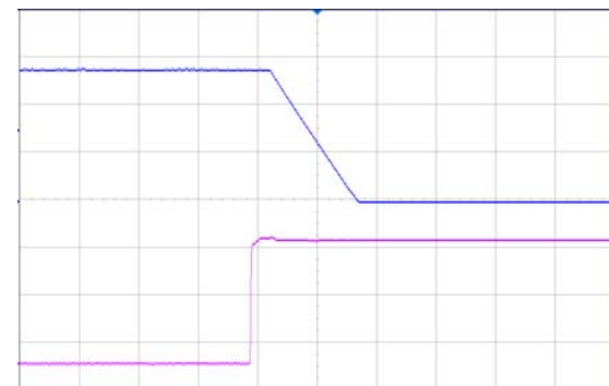
Figure 8 Output voltage shutdown by remote OFF, (1ms/div), see Figure 10 for test configuration; CH1-output voltage (10V/div); CH2-remote OFF voltage (2V/div)
