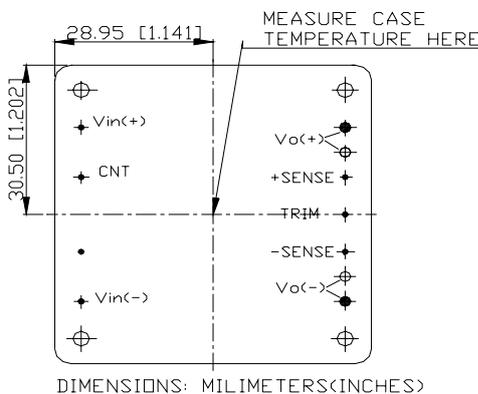
Figure 19 Temperature measurement location (with baseplate)
