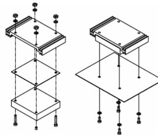
Figure 27 Heatsink mounting
