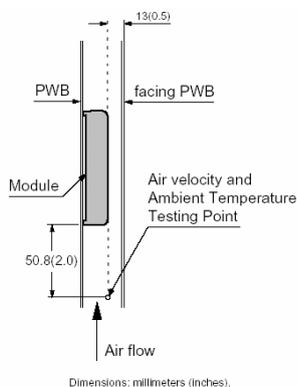
Figure 21 Experiment setup
