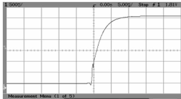
Fig.7 AVE300-48S3V3B-4 Typical Start-up from CNT On
