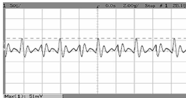
Fig.3 AVE300-48S3V3B-4 Typical Output Ripple Voltage
