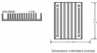
Figure 25 Longitudinal fins heatsink
