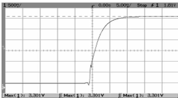
Fig.6 AVE300-48S3V3B-4 Start-up from power on
