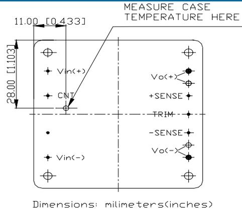
Figure 20 Temperature measurement location (without baseplate)
