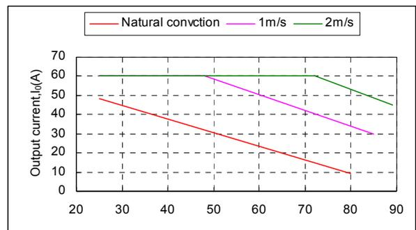
Figure 22 Forced convection power derating without heatsink
