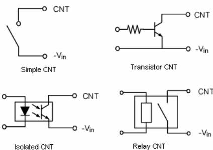
Fig.8 CNT circuits
