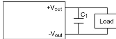
Figure 12 Output ripple filter
