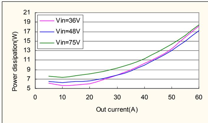
Fig.2 Typical power dissipation curve of AVE300-48S3V3B-4
