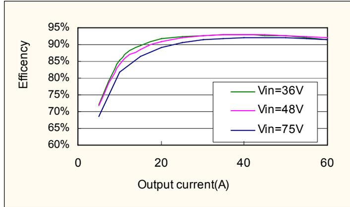
Fig.1 AVE300-48S3V3B-4 Typical Efficiency
