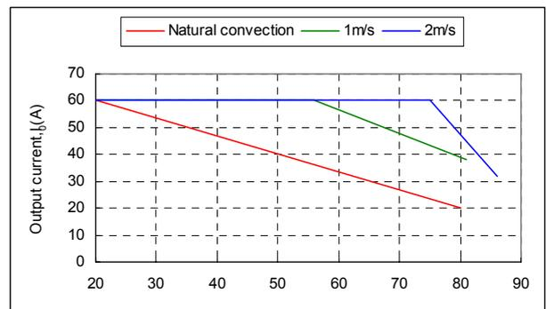
Figure 23 Forced convection power derating without heatsink
