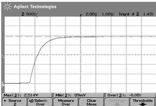
Fig3 AVE300-48S2V5-4 Typical Transient Response to Ta:25°C, Air velocity: 300LFM, forced air direction: from Vin+ to Vin-. Vin: 48V, Vonom, 25% Ionom step from 50% Ionom, 0.1A/µs”, the external capacitor should be “10µ tantalum(ESR≤100 mΩ) // 1µ ceramic capacitor.
