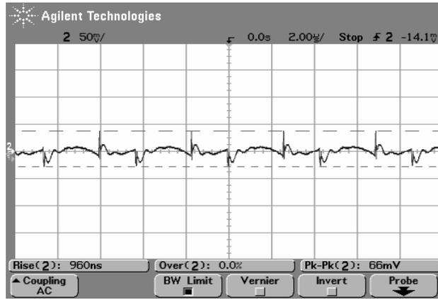
Fig.2 AVE300-48S2V5-4 Typical Output Ripple Voltage
