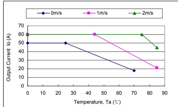
Figure 21 Forced convection power derating without baseplate
