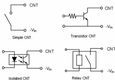
Fig.7 CNT circuits
