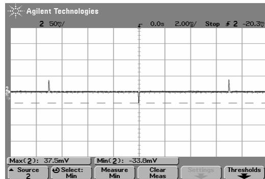
Fig4 AVE300-48S2V5-4. Typical Transient Response to Ta:25°C, Air velocity: 300LFM, forced air direction: from Vin+ to Vin-. Vin: 48V, Vonom, 50% Ionom from 75% Ionom, 0.1A/µs”, the external capacitor should be “10µ tantalum(ESR≤100 mΩ) // 1µ ceramic capacitor.
