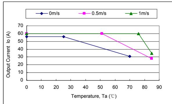
Figure 22 Forced convection power derating with baseplate
