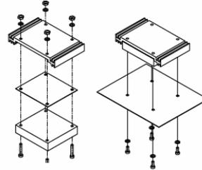
Figure 26 Heatsink mounting
