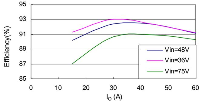
Fig.1 AVE300-48S2V5-4 Typical Efficiency
