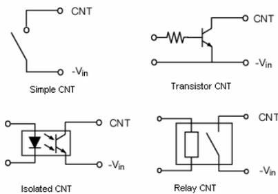
Fig.7 CNT circuits
