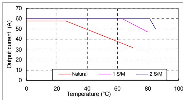
Figure 22 Forced convection power derating with baseplate
