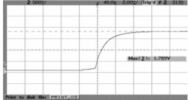
Fig.6 typical start-up from CNT on
