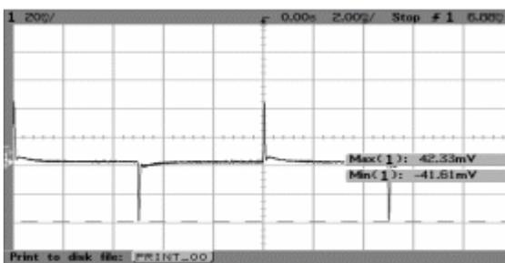
Fig3 AVE300-48S1V8-4 Typical Transient Response to Ta:25°C, Air velocity: 300LFM, forced air direction: from Vin+ to Vin-. Vin: 48V, Vonom, 25% Ionom step from 50% Ionom, 0.1A/μs, the external capacitor should be “10μ tantalum(ESR≤100 mΩ) // 1μ ceramic capacitor.
