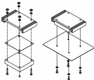
Figure 26 Heatsink mounting
