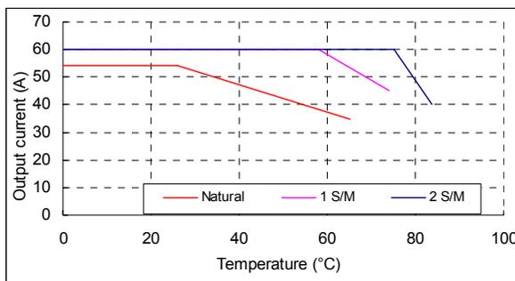
Figure 21 Forced convection power derating without baseplate.
