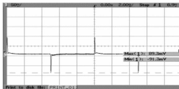
Fig4 AVE300-48S1V8-4. Typical Transient Response to Ta:25°C, Air velocity: 300LFM, forced air direction: from Vin+ to Vin-. Vin: 48V, Vonom, 50% Ionom step from 75% Ionom, 0.1A/μs, the external capacitor should be “10μ tantalum(ESR≤100 mΩ) // 1μ ceramic capacitor.
