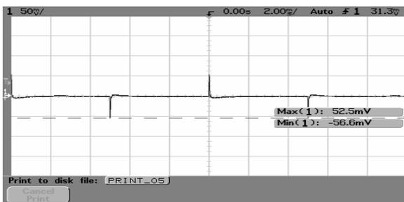
Fig3 AVE300-48S1V5-4 Typical Transient Response to Ta:25°C, Air velocity: 300LFM, forced air direction: from Vin+ to Vin-. Vin: 48V, Vonom, 25% Ionom step from 50% Ionom, 0.1A/μs”, the external capacitor should be “10μ tantalum(ESR≤100 mΩ) // 1μ ceramic capacitor.
