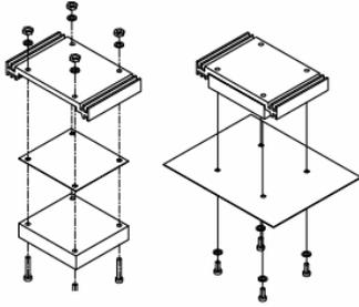
Figure 26 Heatsink mounting
