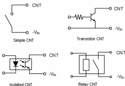
Fig.7 CNT circuits
