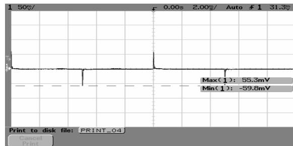
Fig4 AVE300-48S1V5-4. Typical Transient Response to Ta:25°C, Air velocity: 300LFM, forced air direction: from Vin+ to Vin-. Vin: 48V, Vonom, 50% Ionom step from 75% Ionom, 0.1A/μs”, the external capacitor should be “10μ tantalum(ESR≤100 mΩ) // 1μ ceramic capacitor.
