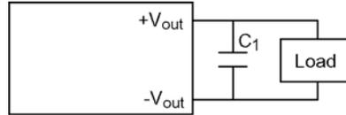
Figure 11 Output ripple filter
