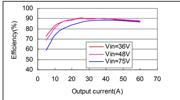
Fig.1 AVE300-48S1V5-4 Typical Efficiency
