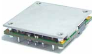
Industry Standard Half Brick: 2.4"X 2.28" X 0.5"
