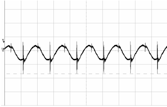
Figure 3 Output ripple & noise (2 \mu s/div, 20mV/div), see Figure 15 for test configuration
