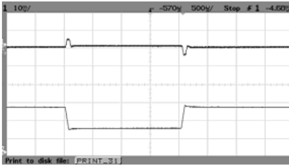
Fig.13 AGQ100-48S2V5 typical transient response to step decrease in load from 50% to 25%, room temperature, 48Vdc input ( \Delta I_o/\Delta t = 0.1A/1\mu s )
