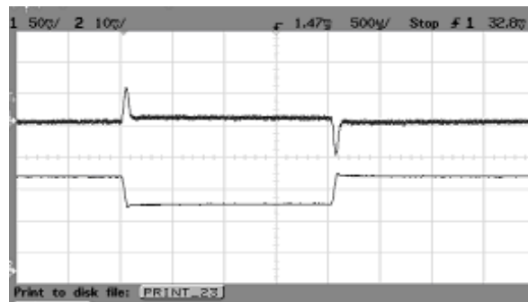
Fig. 18 AGQ100-48S05 typical transient response to step increase in load from 50% to 75%, room temperature, 48Vdc input ( \Delta I_o/\Delta t = 0.1A/1\mu s )
