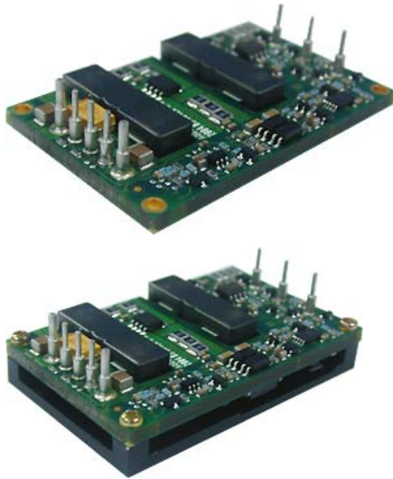
Industry Standard Quarter Brick: 2.28" × 1.45" × 0.4" (open frame) or 2.28" × 1.45" × 0.5" (baseplated)
