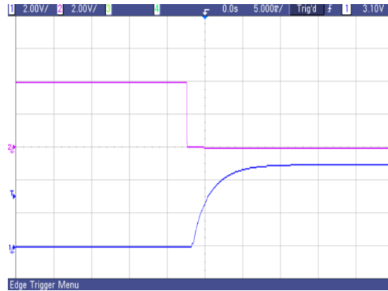
Fig.30 Typical start-up from CNT on of AVQ100B-48S05
