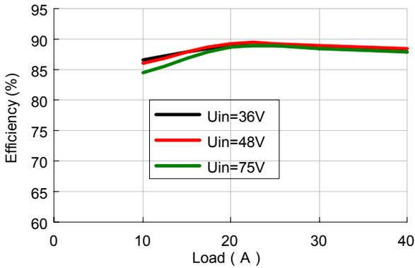
Figure 1 Typical efficiency of AVO100-48S1V5
