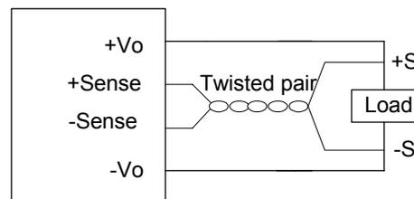
Figure 12 Sense connections
