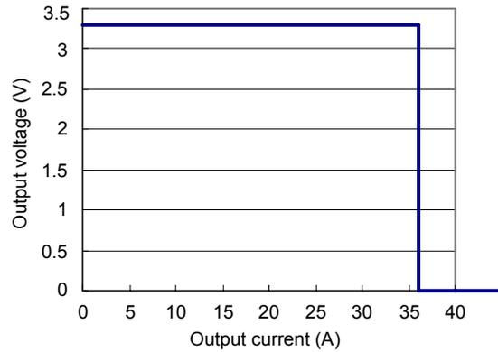
Figure 2 Typical output over-current AVO100-48S1V5
