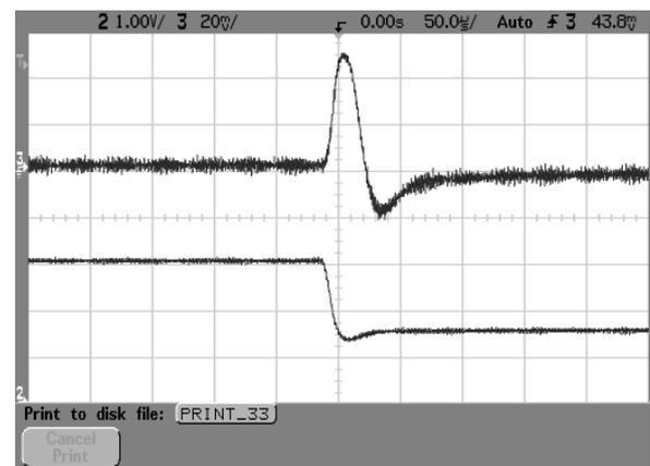
Figure 10 AVO100-48S1V5 typical transient response to step decrease, load change from 50% to 25% of full load, room temperature, 48Vdc Input, ( $\Delta I_o/\Delta t=1A/1\mu s$ ), room temperature,  $I_o=I_{o,max}$
