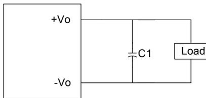
Figure 15 Output ripple filter
