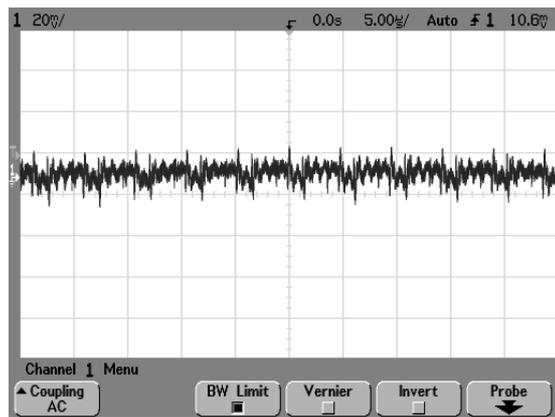
Figure 4 Typical output ripple voltage AVO100-48S1V5
