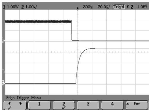
Fig. 6 AVO100-48S1V5 typical start-up from CNT on
