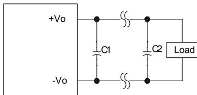
Figure 16 Output ripple filter for a distant load
