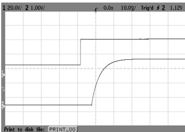
Fig. 5 AVO100-48S1V5 typical start-up from power on
