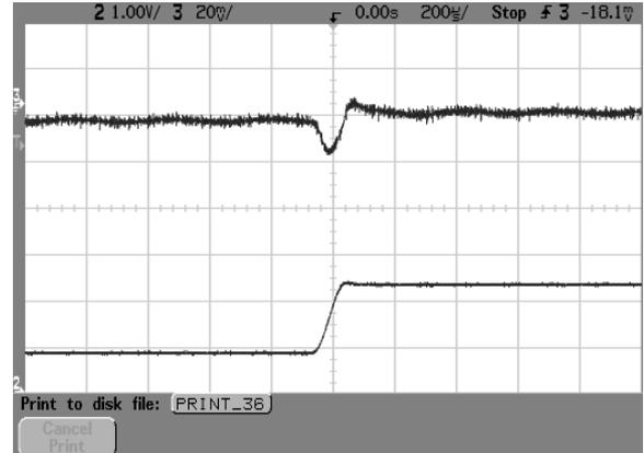
Figure 8 AVO100-48S1V5 typical transient response to step increase, load change from 50% to 75%, of full load room temperature, 48Vdc Input, ( $\Delta I_o/\Delta t=0.1A/1\mu s$ )
