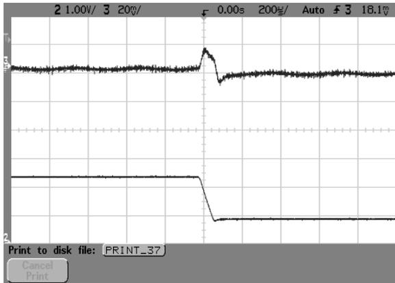
Figure 7 AVO100-48S1V5 typical transient response to step decrease, load change from 50% to 25%, of full load room temperature, 48Vdc Input, ( $\Delta I_o/\Delta t=0.1A/1\mu s$ )
