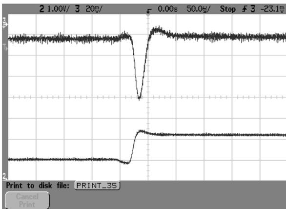
Figure 9 AVO100-48S1V5 typical transient response to step increase, load change from 50% to 75% of full load, room temperature, 48Vdc Input, ( $\Delta I_o/\Delta t=1A/1\mu s$ ), room temperature,  $I_o=I_{o,max}$
