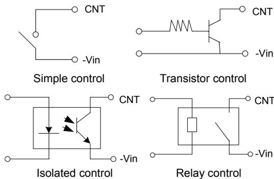
Figure 11 CNT circuits
