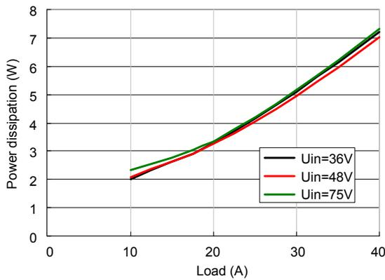
Figure 3 Typical power dissipation AVO100-48S1V5
