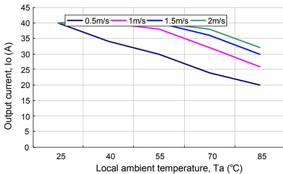
Figure 23 AVO100-48S1V5 output power derating, airflow direction from -Vin to +Vin;  $V_{in}=48V$
