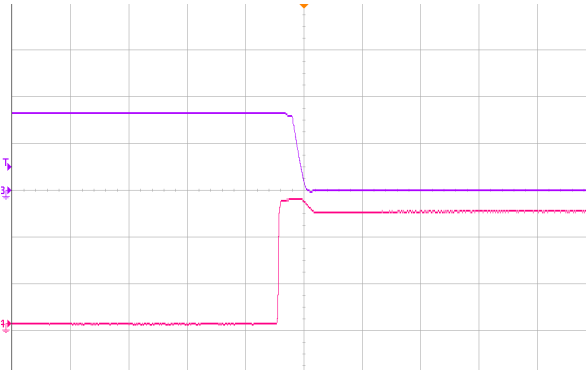
Figure 9 Output voltage shutdown by remote OFF, (500µs/div), see Figure 11 for test configuration; CH4-remote ON (2V/div); CH3-output voltage (2V/div)
