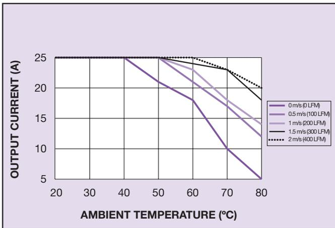
**Figure 7 - Thermal De-rating Curve**
