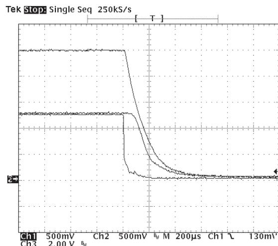
Figure 3 - Typical Response to OUTEN being disabled (Chan1: OUTEN, Chan2:  $V_{ddq}$ , Chan3:  $V_{tt}$ )
