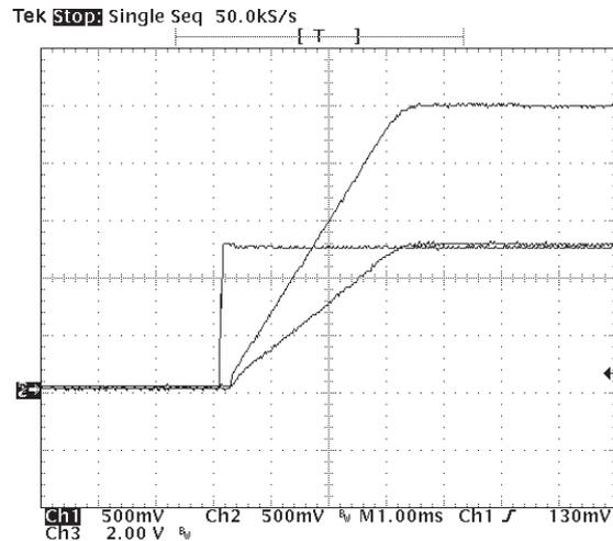
Figure 2 - Typical Response to OUTEN being enabled (Chan1: OUTEN, Chan2:  $V_{ddq}$ , Chan3:  $V_{tt}$ )
