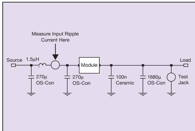
**Figure 9 - Set-up for Measuring Input Ripple Current and Output Ripple Voltage**
