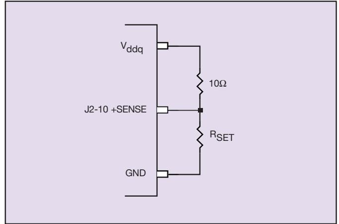
**Figure 8 - Voltage Divider Network for Trimming  $V_{ddq}$  Output**
