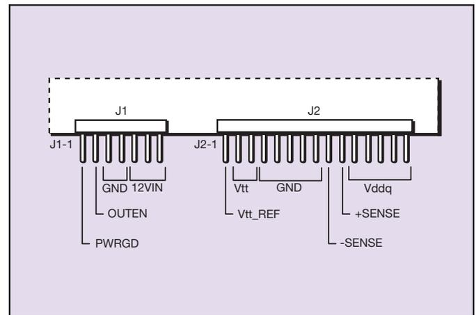
Figure 5 - Pin Diagram for the DDR12
