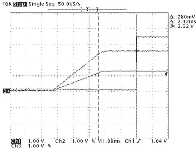
Figure 4 - Power Good Signal being pulled high by external 3.3V source
