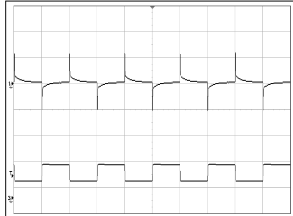
Figure 8: AVD75-48S1V2 Transient Response (1mS/div) 25%-50%-25% load change, 1A/uS slew rate, Ch 1: Vout (50mv/div) Ch 2: Iout (10A/div)
