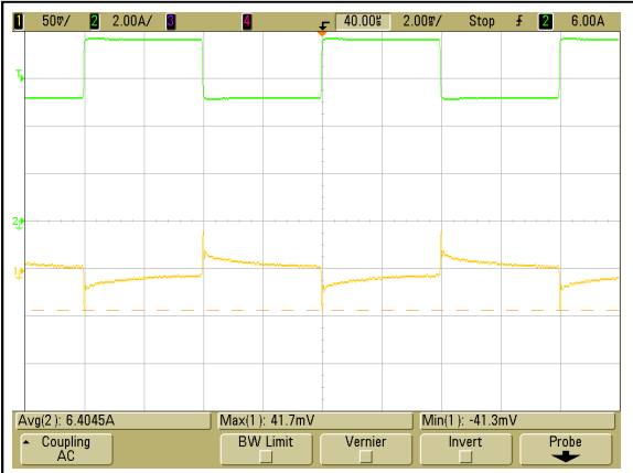
Figure 7: AVD50B-48S05 Transient Response (2mS/div) 0.1A/uS slew rate Ch 1: Vo (50mV/div) Ch 2: Io (2A/div)
