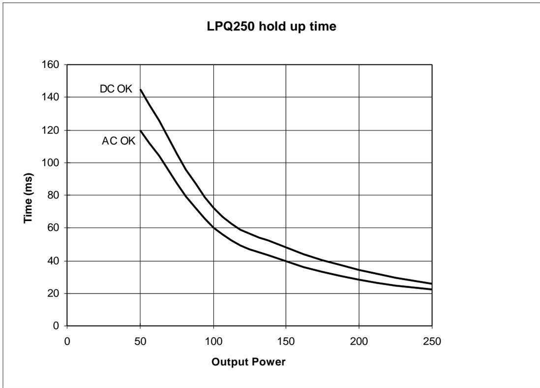
Power supply hold up time is shown by the DC OK line above. The delay time between AC OK and DC OK signals changing state can be seen from the graph above.
