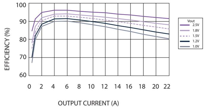
Figure 2 - Efficiency vs Load Current
