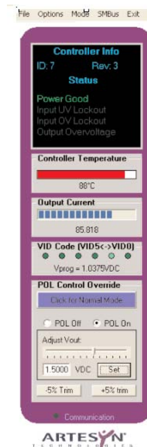
Figure 13 - Typical Computer Display Using the Artesyn Smart SMBus Controller (not part of the AMD VRM) Showing Some of the Features.
