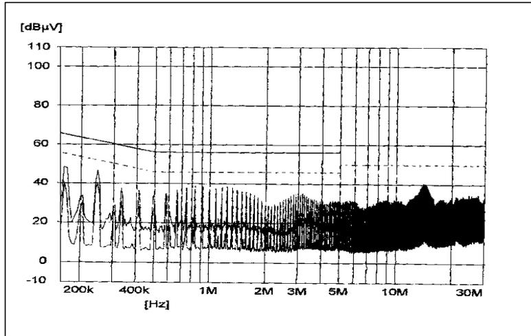
**Fig. 3.** Plot of MVP Conducted Emissions showing Curve B limits of EN55022
