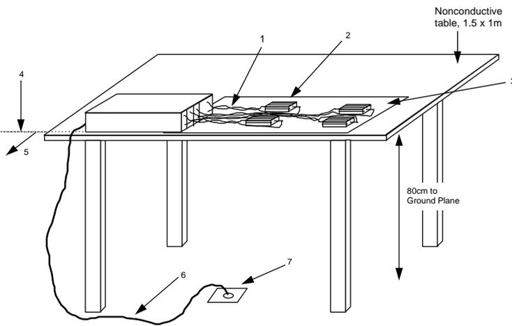
1. Interconnecting cables between output and load are twisted together for each output and then all output interconnections bundled together forming a bundle 1m long.
