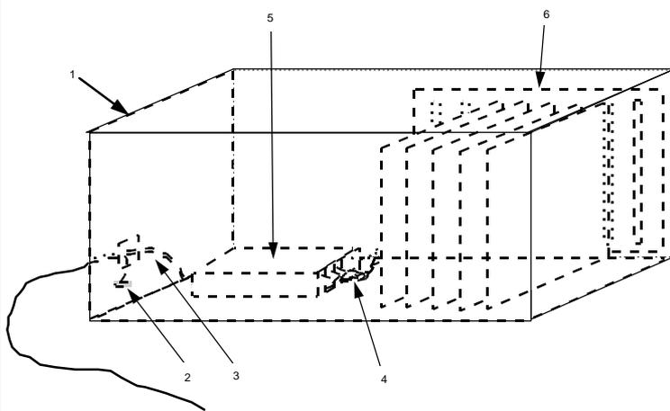
1. Increased attenuation of the radiated emissions can be achieved by careful design of the apparatus enclosure.
