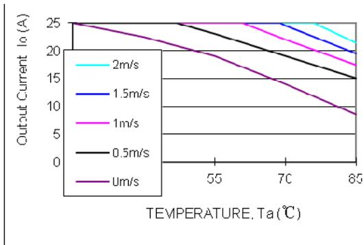
Fig.47 Output power derating AVQ100B-48S3V3
