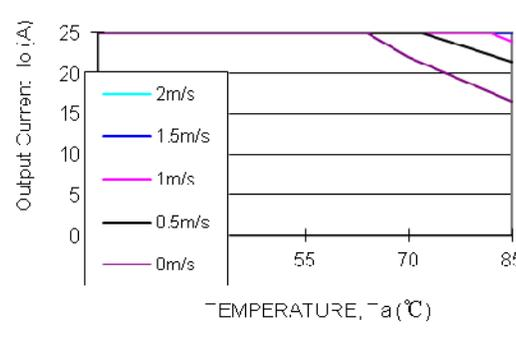
Fig.44 Output power derating AGQ100-48S1V5
