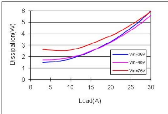
Fig. 11 Typical power dissipation curve of AGQ100-48S1V2
