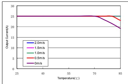
Fig.45 Output power derating AGQ100-48S1V8
