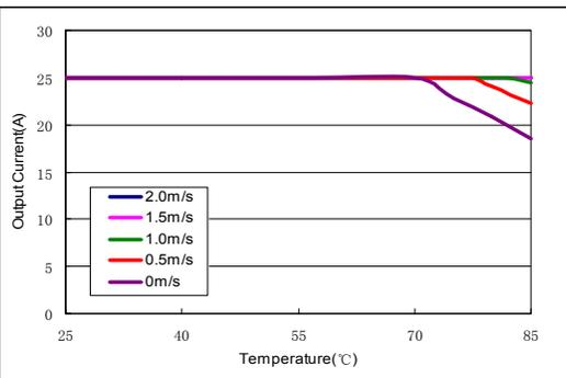
Fig.46 Output power derating AGQ100-48S1V8
