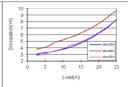
Fig. 14 Typical power dissipation curve of AVQ100B-48S3V3
