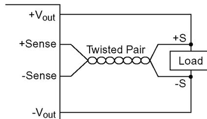
Fig. 52 Sense connections
