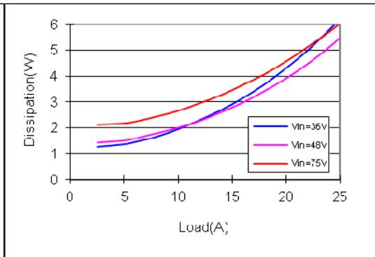
Fig. 12 Typical power dissipation curve of AGQ100-48S1V5
