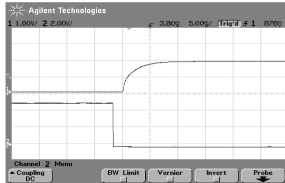
Fig.26 Typical start-up from CNT on of AGQ100-48S1V8
