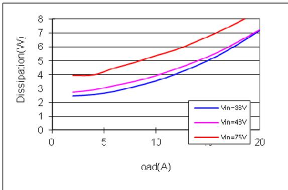
Fig. 15 Typical power dissipation curve of AVQ100B-48S05
