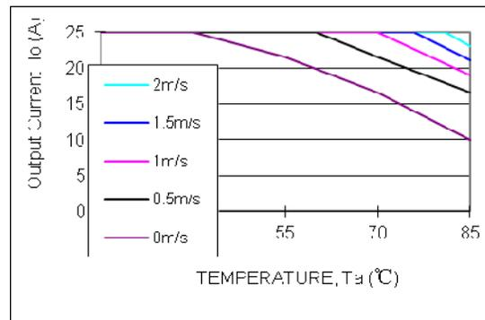
Fig.48 Output power derating AVQ100B-48S3V3
