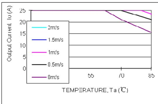
Fig.43 Output power derating AGQ100-48S1V5
