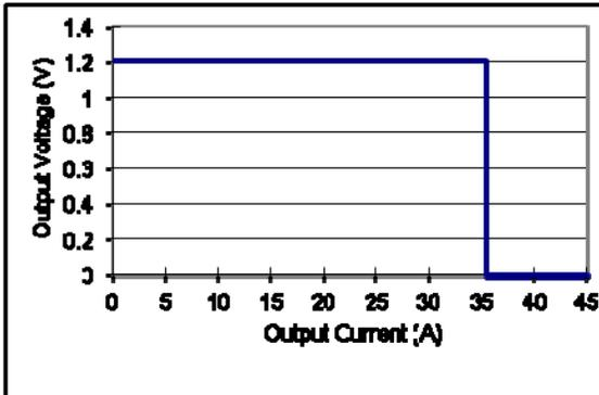
Fig. 6 Typical over-current of AGQ100-48S1V2
