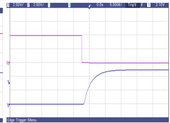
Fig.30 Typical start-up from CNT on of AVQ100B-48S05
