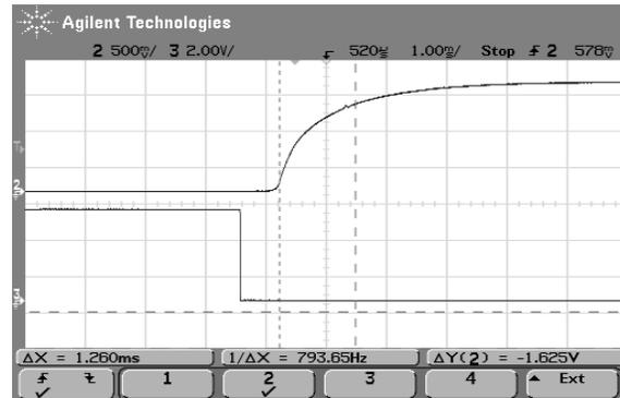
Fig.24 Typical start-up from CNT on of AGQ100-48S1V5
