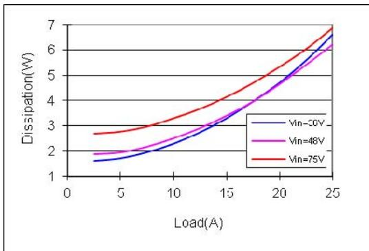
Fig. 13 Typical power dissipation curve of AGQ100-48S1V8
