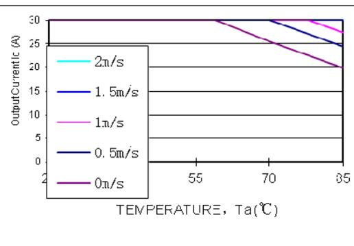
Fig.42 Output power derating AGQ100-48S1V2
