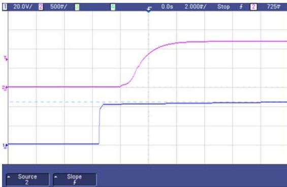
Fig.21 Typical start-up from power on of AGQ100-48S1V2
