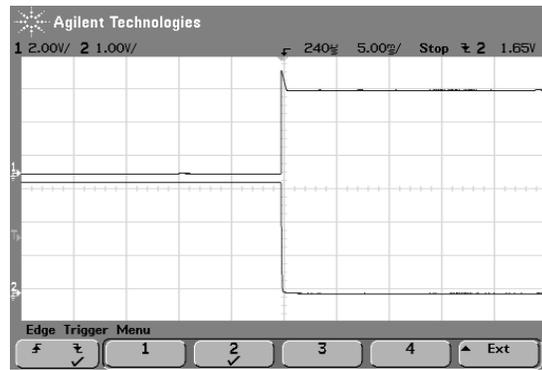
Fig.28 Typical start-up from CNT on of AVQ100B-48S3V3
