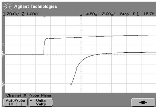
Fig.27 Typical start-up from power on of AVQ100B-48S3V3
