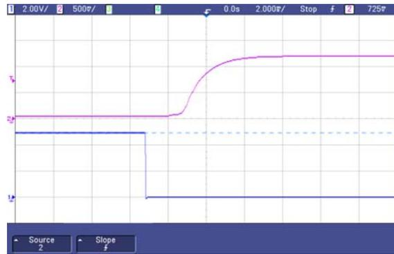
Fig.22 Typical start-up from CNT on of AGQ100-48S1V2
