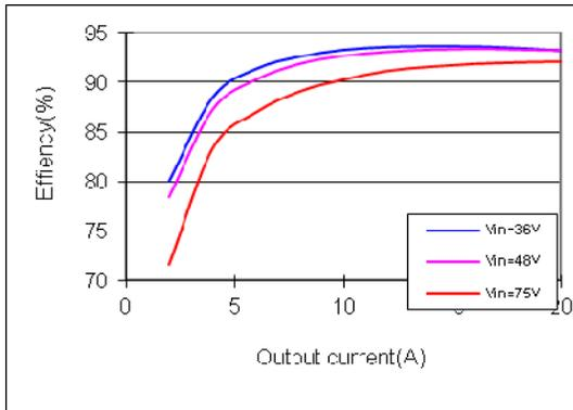
Fig. 5 Typical efficiency of AVQ100B-48S05
