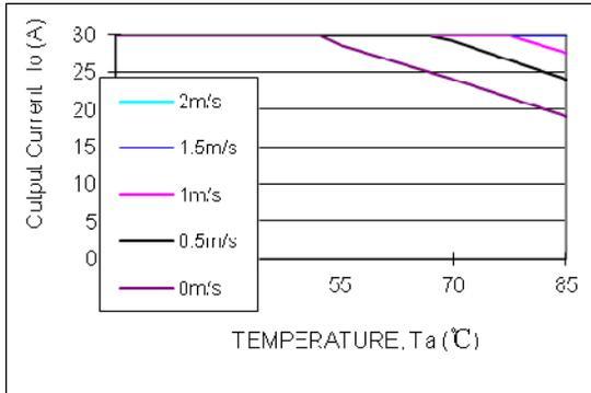
Fig.41 Output power derating AGQ100-48S1V2
