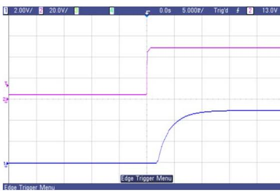
Fig.29 Typical start-up from power on of AVQ100B-48S05
