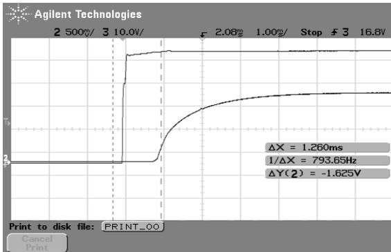
Fig.23 Typical start-up from power on of AGQ100-48S1V5
