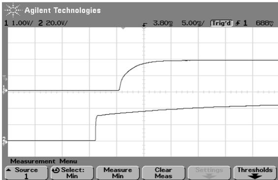
Fig.25 Typical start-up from power on of AGQ100-48S1V8
