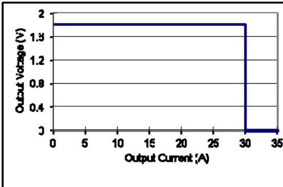
Fig. 8 Typical over-current of AGQ100-48S1V8
