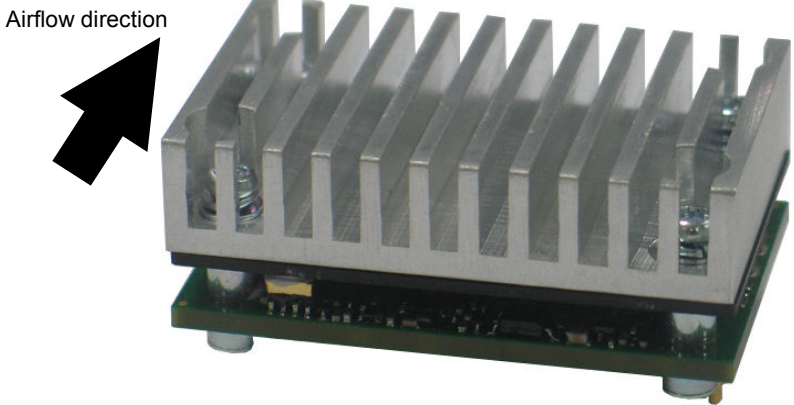
Figure 17 Typical test condition, heatsink size (L x W x H): 57.9mm x 36.8mm x 6.3mm
