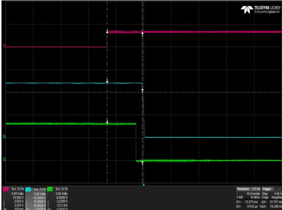
Figure 7: DS500SPE-3 Turn Off Characteristic via PS_ON_L Full Load: I_o = 38.7A , I_{SB} = 3A Ch 2: PS_ON_L Ch 3: V_o Ch 4: Pwr_Good
